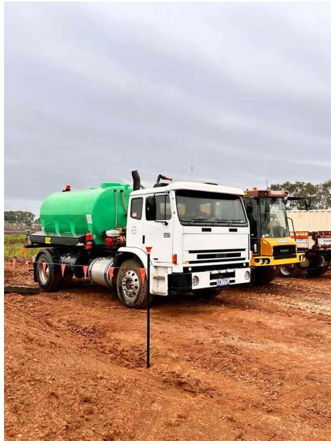
Photo B22-1: Water carts available on site to suppress dust
