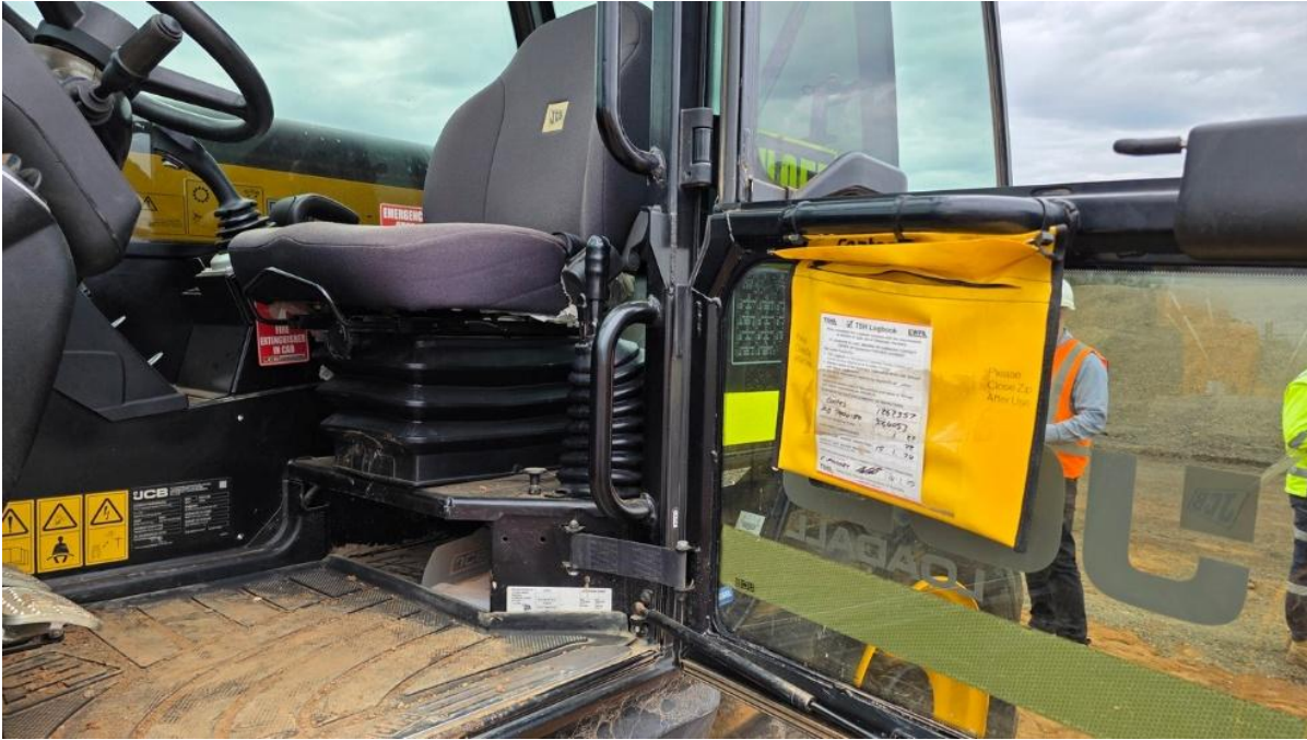
Photo A10-1: Mobile plant equipped with fire-extinguishers appropriately tagged. Service history demonstrating mechanical and safety checks performed
